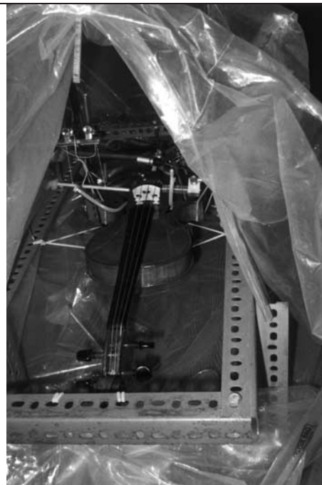
Figure 1. (a) General view of the experimental setup with the glove bag. The violin is turned upside-down for measurements in He(5N). (b) Typical setup inside the glove bag showing transducers mounted on the violin with acoustic exciter and microphone tubes passing into f -holes, impulse pendulum and magnet/coil at the bridge, and microphone above the violin.
